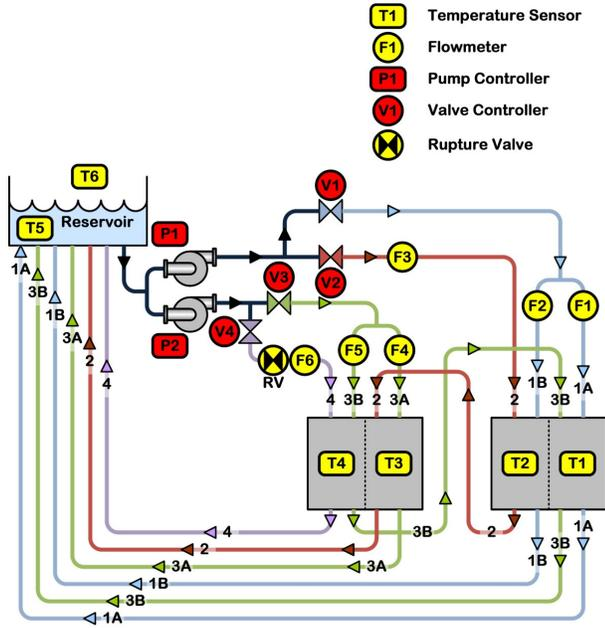
Figure 2. Architectural overview of the chilled water plant demonstrator.
