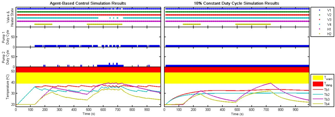
Figure 5. Agent-based control versus 10% constant duty cycle simulation results
