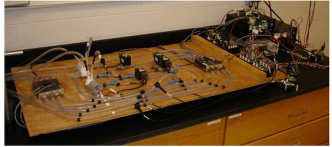
Figure 3. Fully constructed chilled water demonstrator system.
