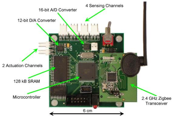
Figure 1. Narada wireless node for shipboard plant monitoring and control.
