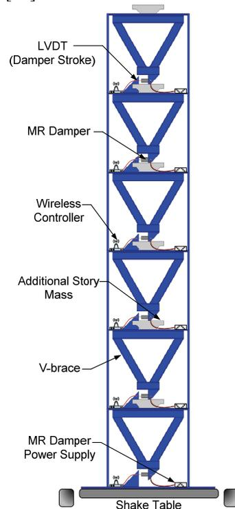
Fig. 1. 6-story partial-scale single-bay steel structure used for validation of MR damper control laws on the NCEE shake-table.
