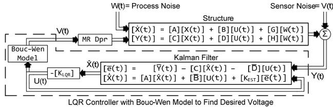
Fig. 3. Block diagram of LQG control of MR dampers.
